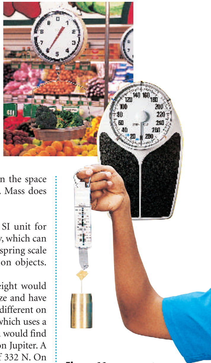
Figure 11 A spring scale measures an object's weight by how much it stretches a spring.
