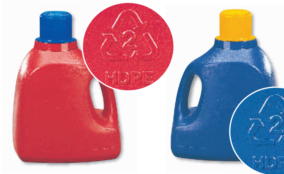
Figure 2 The identity of the material does not necessarily depend on its color. Each of these bottles is made of high-density polyethylene (HDPE).
