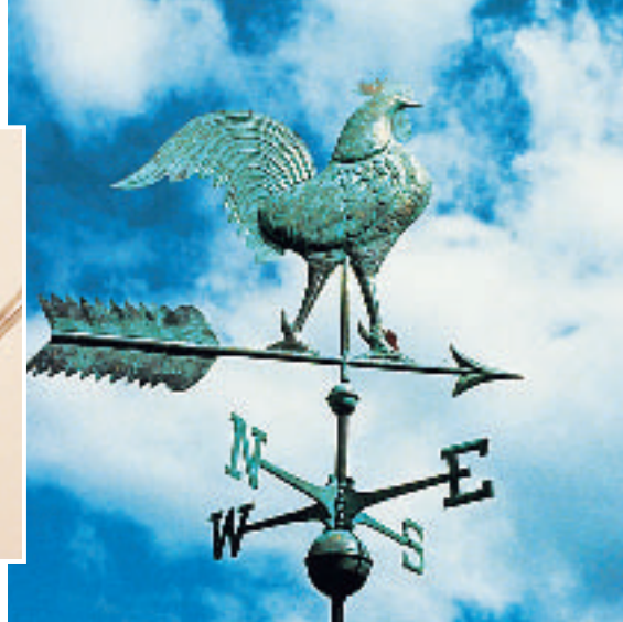
Figure 13 Many kinds of interactions with oxygen can occur. Copper sculptures develop a green patina, which is a mixture of copper compounds.
