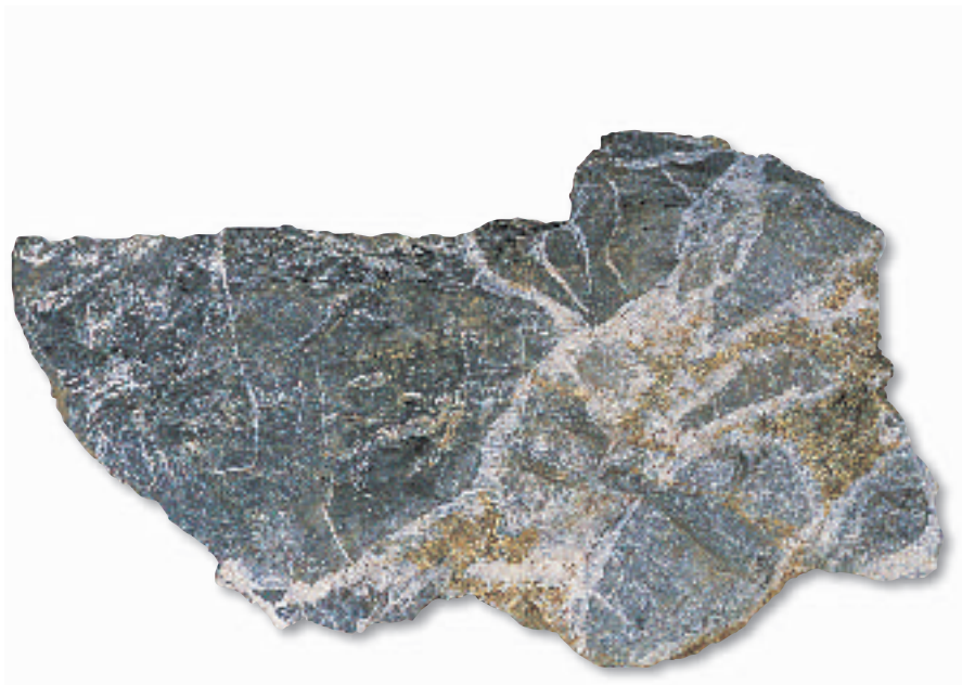
Figure 15 The mineral sphalerite (greenish when nearly pure) is an important source of zinc. Iron often is coated with zinc to prevent rust in a process called galvanization.
