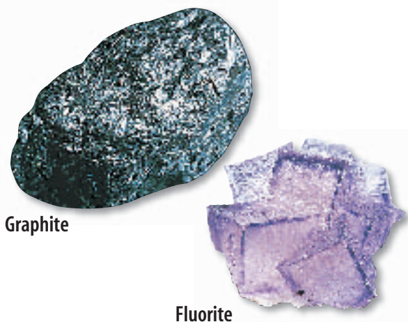
Figure 8 Luster is an important physical property that is used to distinguish minerals. Graphite has a metallic luster. Fluorite has a nonmetallic, glassy luster.
