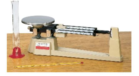
**Figure 11** Some of the equipment used by scientists is shown here. A graduated cylinder is used to measure liquid volume. Mass is measured with a balance. A scientist would use a thermometer with the Celsius scale to measure temperature.
